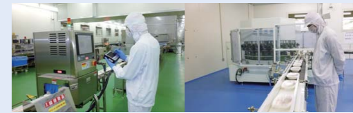
Controlling the activity of workers by using different floor colors to indicate different levels of sanitary protection.
