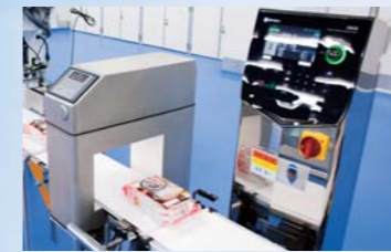
X-ray inspection device to detect foreign objects: All images are stored so as to enable a follow-up investigation when necessary.
