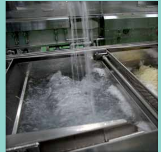
Cooling boiled 'UDON' noodles as part of the production process
